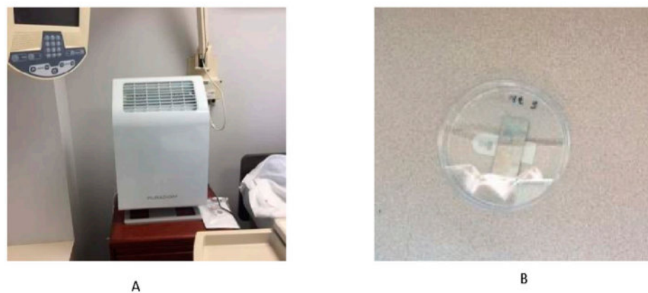
Figure 1. The photocatalytic reactor setup in the hospital room. (A) The photocatalytic reactor. (B) Sterile stainless steel carriers were individually placed in sterile petri dishes and affixed to the bottom of each petri dish with adhesive and placed at multiple locations.
